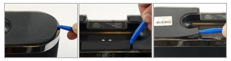
Remove the rubber from the bottom of the speaker, use a medium blue plastic spudger to gently work its way under the rubber and slowly peel off for each of the three feet. The order does not matter.
