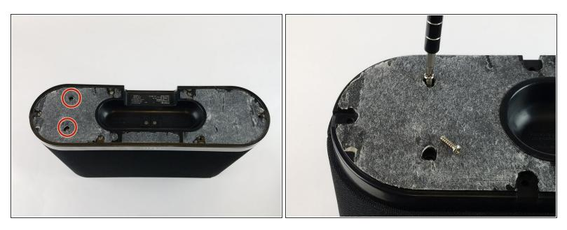
• Remove the two remaining 11 mm Philips #1 screws holding the base and set them aside.
