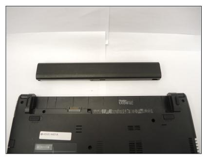
Flip over the laptop and remove the battery for ease of replacement.
