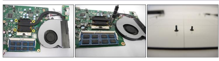
• Flip the motherboard over and you will notice four screws (circled in yellow) that are connecting the fan's bracket to the motherboard. Using your screwdriver, remove the four screws and place them off to the side.
