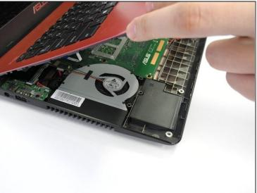
• Flip the laptop back over and begin prying the keyboard cover from the rest of the laptop by using a plastic spudger.
