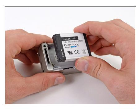
Remove the battery from the case.
