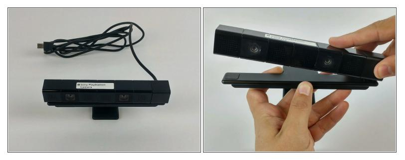
• Separate the camera from the camera stand to gain access to the bottom of the camera.
