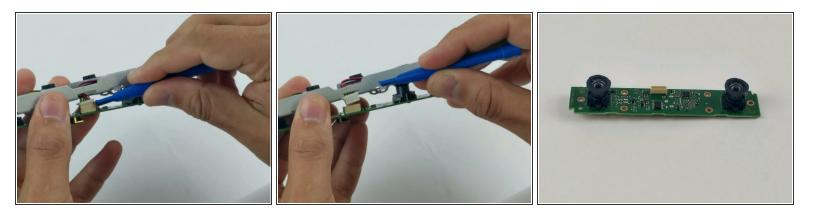
• Using a plastic opening tool, disconnect the microphone array connector from the motherboard.
