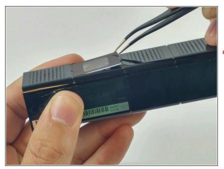
• Using the tweezers, remove both poly-carbonate lens coverplates.
