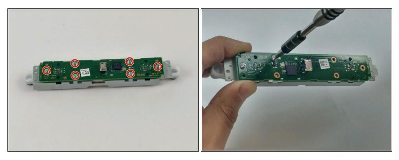
Using the PH0 sized screwdriver, remove the six 4.2mm Phillips #0 screws securing the motherboard to the metal frame.
