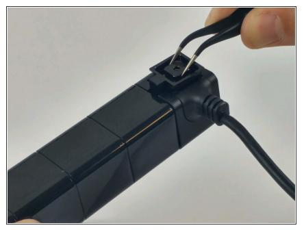
• Using tweezers, remove the cap holding the cable grommet in place.
