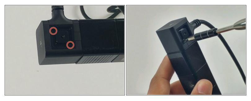
Using a PH000 sized screwdriver, remove the two 6.5mm Phillips #000 screws located under the stand connection point, where the cable enters the case.
