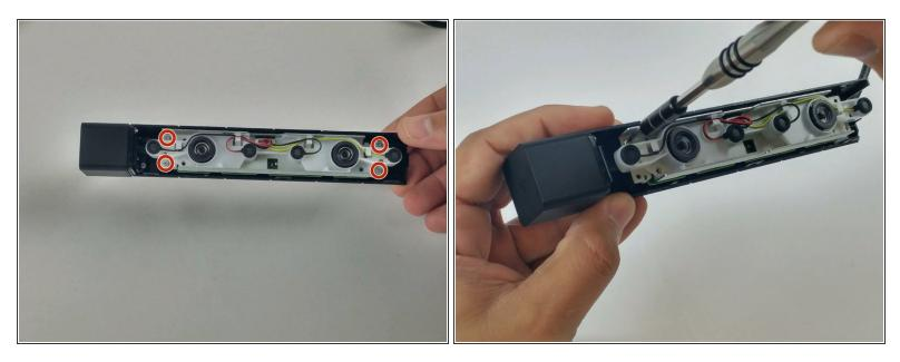
Using the PH0 sized screwdriver, remove the four 4.5mm Phillips #0 screws securing the circuit assembly to the device housing.
