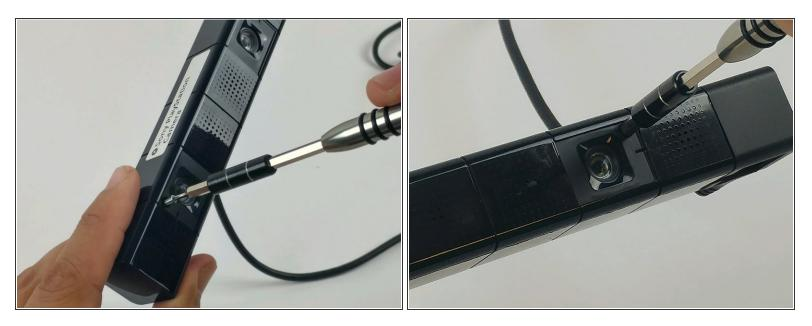
Using the PH0 sized screwdriver, remove two 3.2mm Phillips #0 screws, located under the coverplates.
