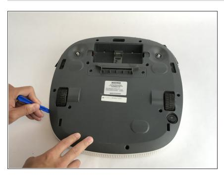
Use spudger or plastic opening tool to separate the Deebot backside
