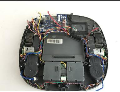
Locate and disconnect 12 cables bundles connected on the motherboard
