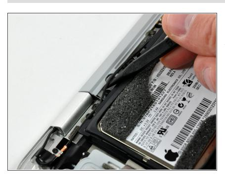
Use the pointed end of a spudger to de-route the microphone cable from the hard drive bracket.
