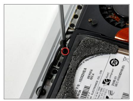
Remove the 4.7 mm Phillips screw securing the hard drive to the upper case.
