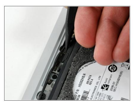
Use the tip of a spudger to remove the cosmetic screw cover to reveal the last remaining screw securing the hard drive.
