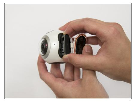
• Once the battery has popped out, pull the battery out of the camera.
