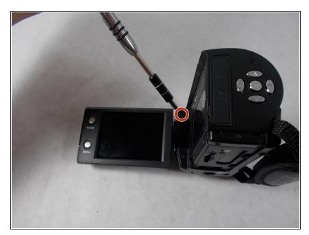
Remove the top screw to the right of the screen.
