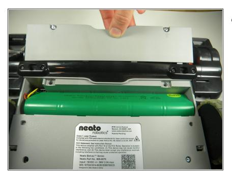
Remove the battery back plate to reveal the battery.
