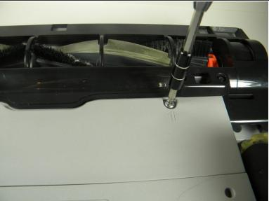
• Use the Phillips #1 screwdriver to loosen both screws.
