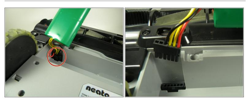
• Disconnect the current battery by pulling the connector from the base and pushing on the clip.
