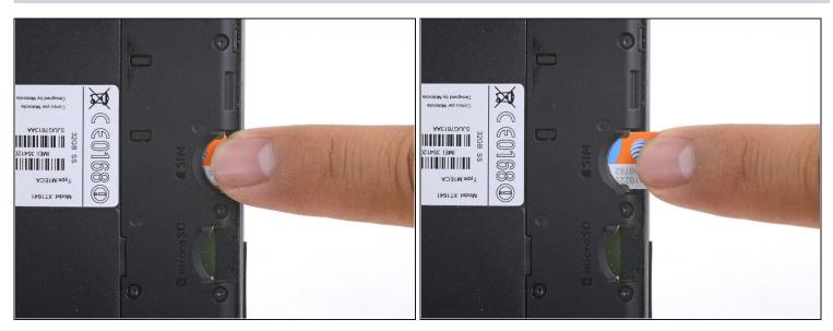
Slide out and remove the SIM card.
