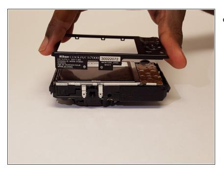
Carefully remove the back frame of the camera.
