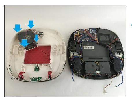
Locate the 4 screws on the vacuum motor.
