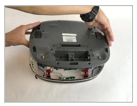
• Carefully lift the back cover from the body of the Deebot to expose the internal wiring harnesses.
