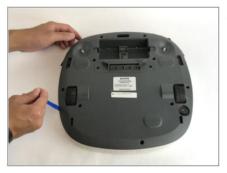
Use a spudger or plastic opening tool to separate the Deebot backside.
