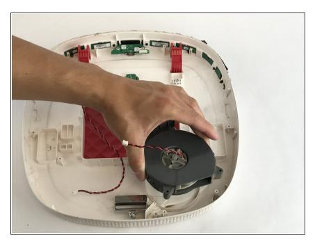
• Remove the vacuum motor body
