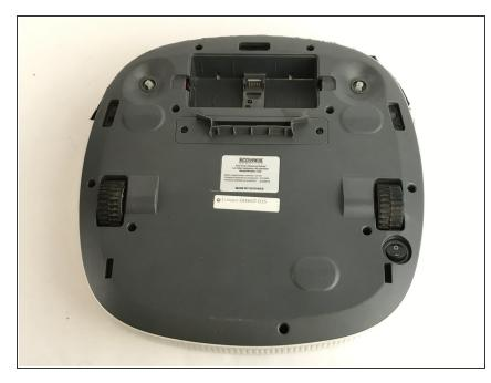
Lay the Deebot face down so you have access to the battery compartment. Remove the battery.
