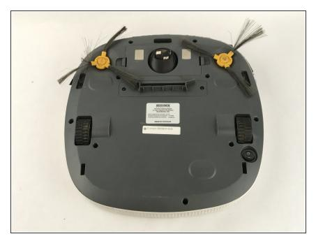
Roll the Deebot over on a flat surface. The brushes will be located on the front with bright yellow connectors.
