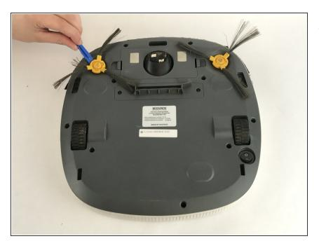
Place a plastic opening tool under the lip of the brush head.
