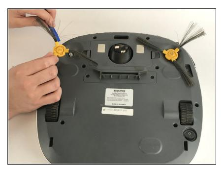
Gently pry up with the opening tool so that the brush comes out completely.
