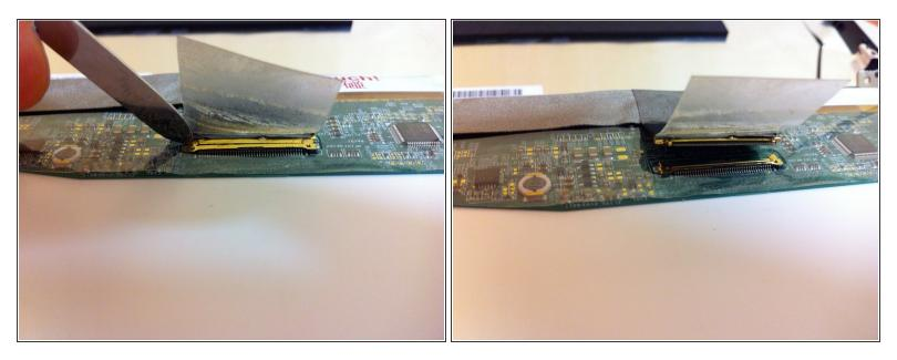
• Carefully disconnect the cable with a spuger.
