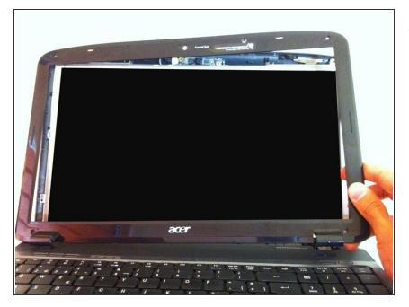
When all the clips are out, the entire plastic frame should come out easily.
