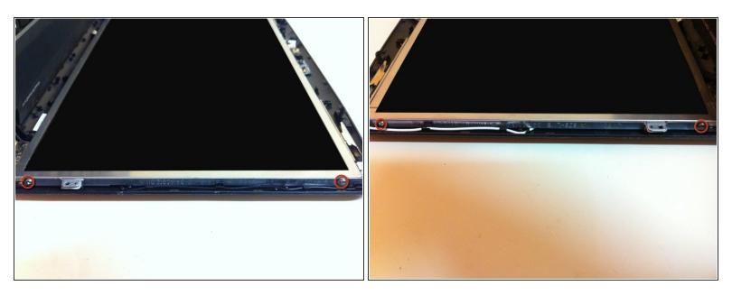
• Remove the 4 screws located in the sides of the LCD screen.
