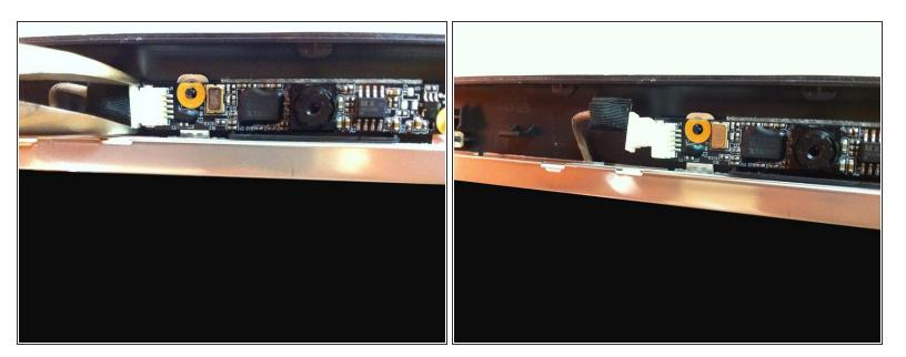
• Carefully disconnect the camera cable.
