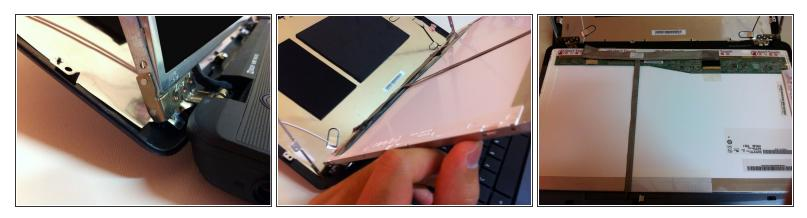
• Take the LCD screen out of the metal frame and flip it towards the keyboard.
