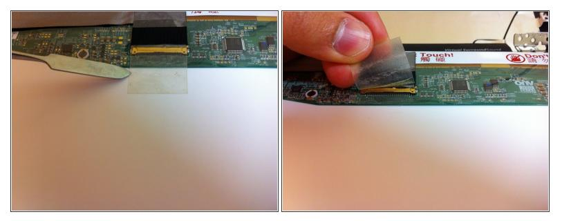
• Remove the tape that holds the display cable.
