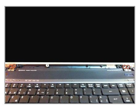
Remove the other 4 screws that secure the metal LCD frame to the hinges.
