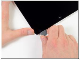
Continue sliding the iSesamo along the left half of the bottom edge of the iPad, releasing the adhesive all the way to the corner.
