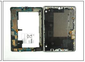
Take the plastic opening tool around the tablet to remove the motherboard from the device.
