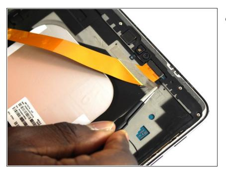
Using the precision tweezers, remove the silver tape that is holding the orange ribbon cable connecting the two pieces.
