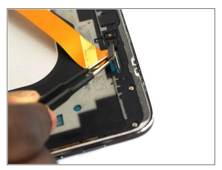
Using the precision tweezers, remove the small press-fit connector from the body of the tablet.
