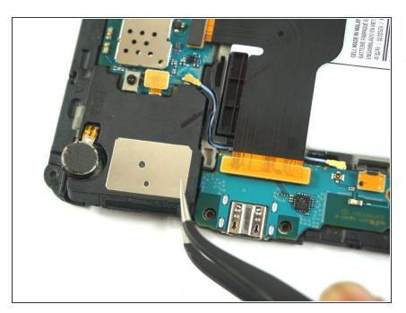
• Using the precision tweezers, remove the speaker.
