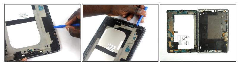
• Take the plastic opening tool around the tablet to remove the motherboard from the device.
