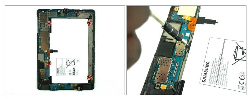
Using the Phillips #000 Screwdriver, remove the four 2.74mm black screws around the edge of the battery.
