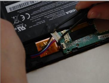
Using needle-nose tweezers, gently push the large white wire connector (connected to the black, red and blue wires) out of its housing.
