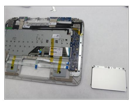
• Slide the trackpad out from underneath the ribbon cables.
