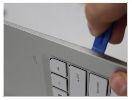
Use the opening tool to carefully remove the back cover of the keyboard.
