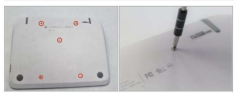
• Use a J1 screwdriver head to remove the remaining 5mm screws at the back of the keyboard part.
