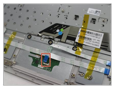
• Disconnect the ribbon cable and move it out of the way.
