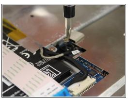
Remove all eight 3mm Phillips screws using a J1 screw head.
