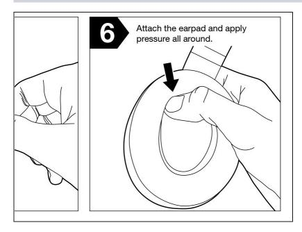
So take your ear pad and align the top dowel to the hole, push it in, and then align the bottom one. Apply pressure on the ear pads for a good minute that way you remove any gaps. If you have noticeable gaps, that means you have not aligned the cushion correctly and try again.
