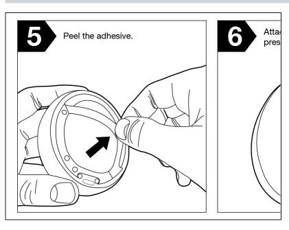
There are two dowels on the headphone, on the top left and the bottom right. You can get a better understanding of how to apply the cushion to the headphones before peeling the adhesive.
