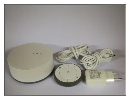
The Gateway I'm tearing down today came from the Ikea Gateway Kit, which includes the Gateway, two bulbs, a remote, a USB A to Micro-B cable, a Ethernet cable and a 5V @ 1A charger.
