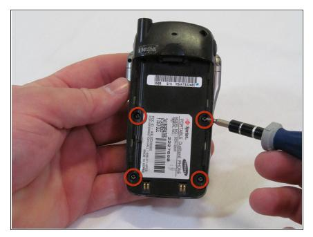
Remove the four screws using a T6 Torx screwdriver.
