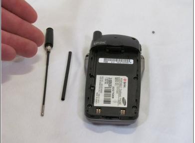
Pull the guide tube free from its retaining ring and slide it out the top.
