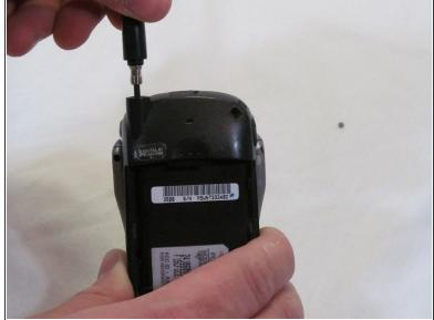
• Grasp the antenna firmly and rotate it counterclockwise to unscrew it from the phone.
