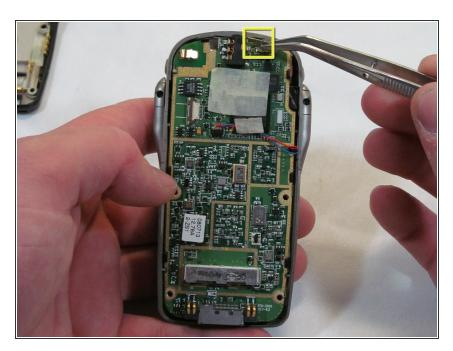
Remove the connector for the earpiece speaker, located on the upper end of the logic board.
