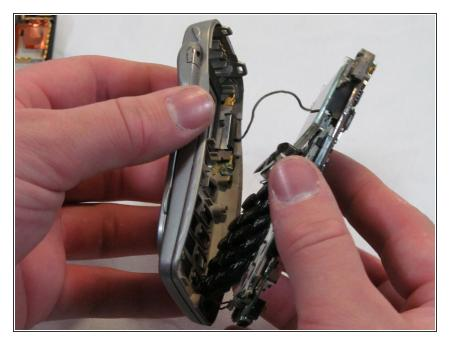
Turn the front cover over, gently prying the logic board away from the front cover. It will remain attached by two wires from the front of the board.
