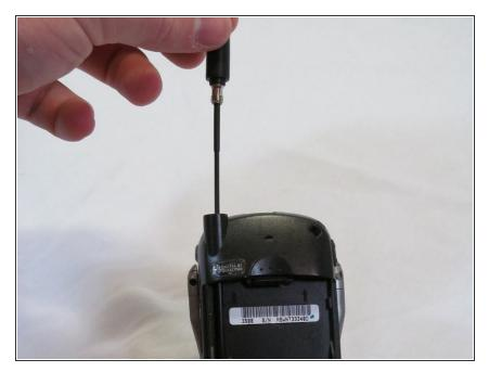
When unscrewed, pull the antenna straight up and out.
