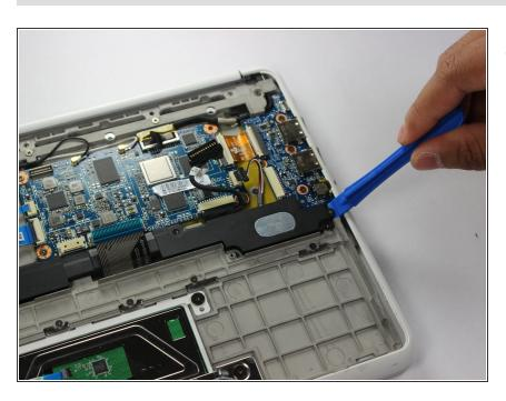
Use the plastic opening tool to remove the speaker from back panel.
