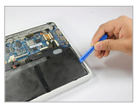
Using the plastic opening tool remove the battery from the Chromebook.
