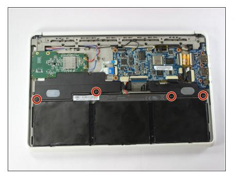
Unscrew the four 1.2mm screws using the Phillips #1 screwdriver.
