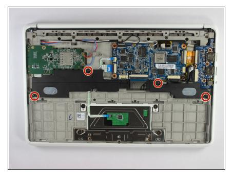
Use the Phillips #1 screwdriver to remove the four 1.2mm screws circled red.
