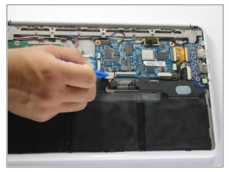
Disconnect the battery input to the motherboard using the plastic opening tool
