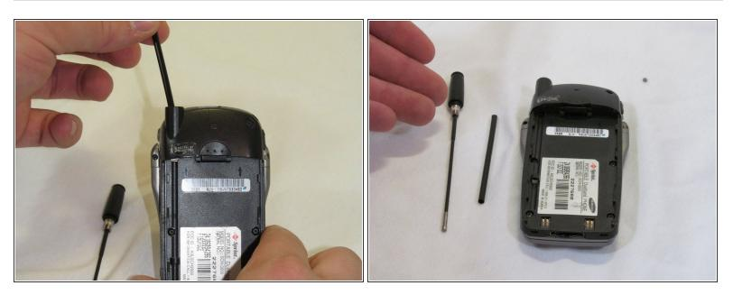
• Pull the guide tube free from its retaining ring and slide it out the top.
