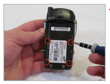
Remove the four screws using a T6 Torx screwdriver.
