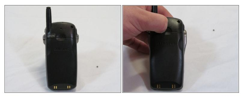
• Place the phone so that the back is facing you. Depress the locking tab on the back of the phone with a finger or thumb.
