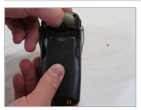
Slide the battery toward bottom of the phone, about a quarter of an inch, to clear the hooks that keep it secured to the back of the phone.
