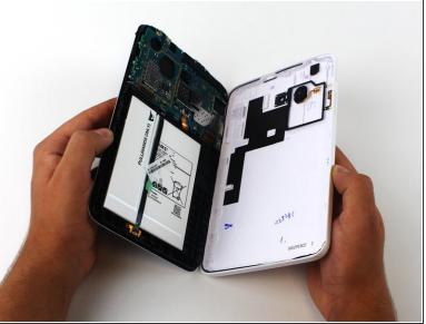
After separating the latches holding the screen and case together, slowly take the screen off the case.
