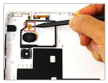
Using a spudger, pry up the speaker ribbon cable.
