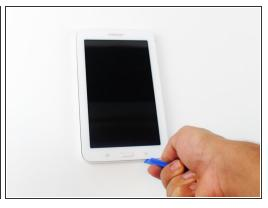
Make sure the device is turned off before attempting to disassemble it.
