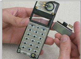
Using your index finger and thumb, carefully remove LCD display screen. You may need to use a
