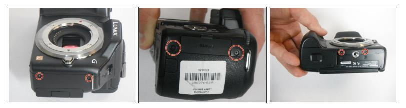
Remove the four 4.6mm J000 Phillips screws from the sides and two 3.2mm J000 Phillips screws along the bottom.
