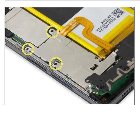
Remove the three Phillips #000 screws on the silver panel.
