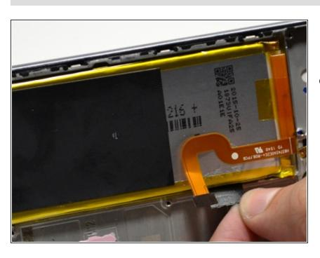
Locate the adhesive strip underneath the battery. Gently pull on the strip to loosen it enough to remove the battery from the device.
