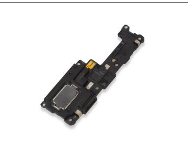
Use the <u>Spudger</u> to gently remove the Loudspeaker from the device. Place the replacement Loudspeaker into the device.
