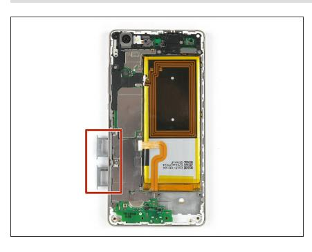
Continue by removing the SIM and SD card trays on the side of the device.
