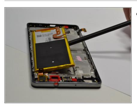
Use the <u>Spudger</u> to gently remove the battery. Then insert the replacement battery.
