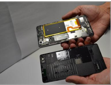
Begin by removing the back cover of the device with the <u>Spudger</u>. To prevent damage to the back cover, begin removing the cover half an inch to the right of the headphone jack and continue prying around the perimeter of the device.
