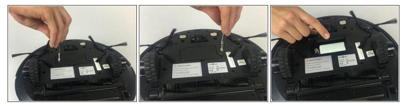
• Remove both screws shown by rotating them counter-clockwise.
