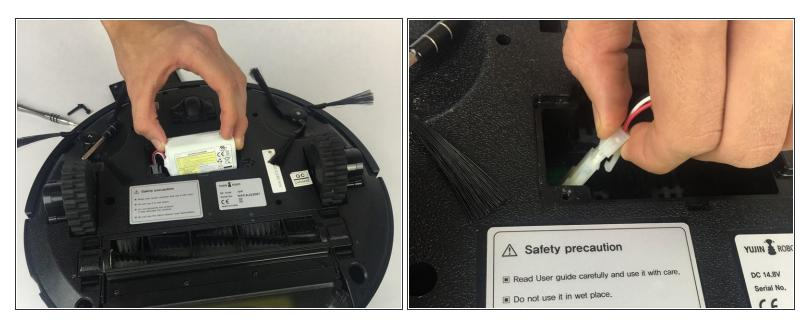
• Slide the battery out, and disconnect it from the robot by squeezing the tab on the power cable.
