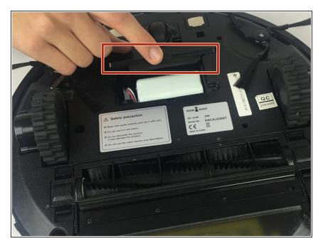
Remove the battery compartment's lid.
