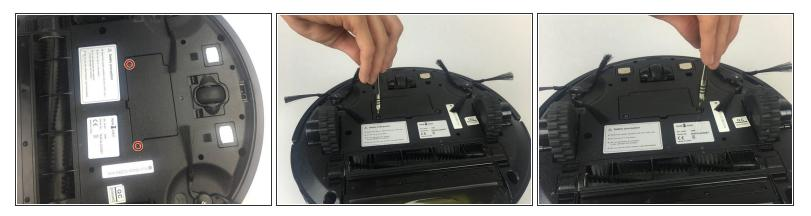
• Locate and unscrew the two 15mm screws with a Phillips #2 screwdriver.
