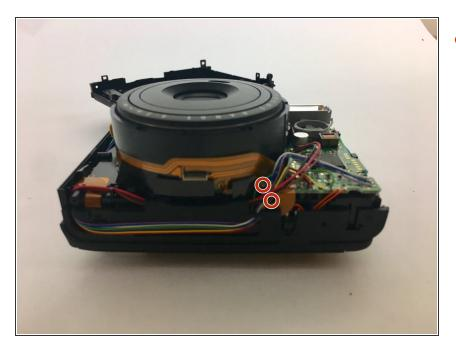
Remove the next two screws with a Phillips #000 screwdriver. The upper screw, sized 1.75 mm, is facing in towards the center of the lens unit. The lower screw, sized 4.75 mm, is to the right of the upper screw and faces down into the camera.
