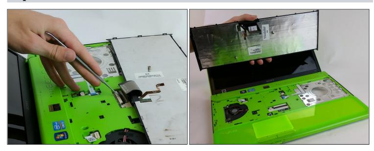
• To fully release the old keyboard, lift the black wedge clip by using the spudger tool to press down on the clip and release the wider cable.
