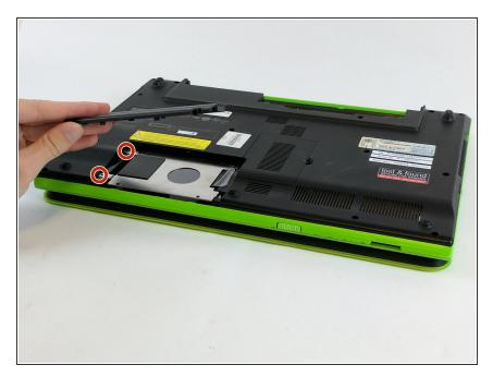
Remove the screws that hold the hard drives metal tray in place. Use a spudger (as seen in the photo) to lift up the hard drive's metal tray.
