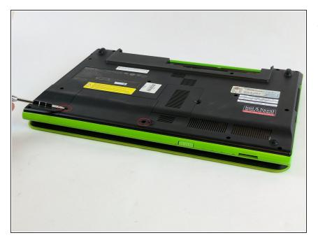
First remove screws from the plastic cover on the bottom of the device using a Phillips head #1 screw driver.
