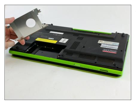
• Remove the metal tray and the hard drive which is attached to it.
