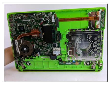
Once screws are removed, remove the back cover.
