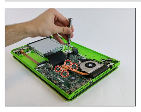
Unscrew the four screws surrounding the heat sink.
