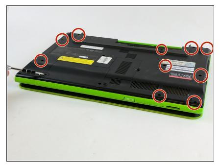
Remove all the screws that hold the plastic bottom cover on. There are some more screws that cant be seen in the photo.
