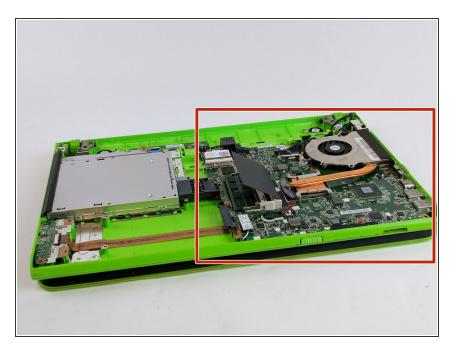
Now that the backing plate is off make sure to be careful of the Motherboard and its components from being damaged. From here on out it is recommended that you wear an anti static bracelet or at the very least touching something metal to remove any static electricity that you may have built up.
