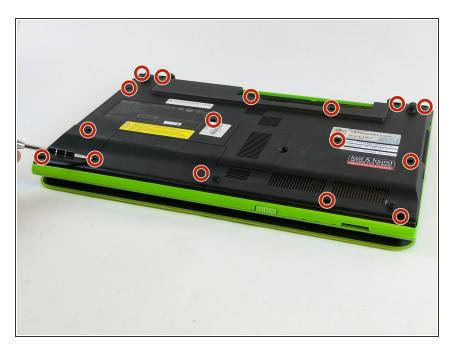
Remove all the screws that hold the plastic bottom on. There are some more screws that can't be seen in the photo.
