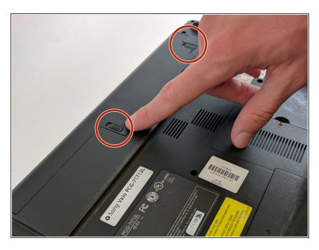
Unlock the battery and push the release lever to remove the battery from the laptop.
