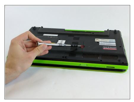
Turn the laptop upside down. Locate a removable cover, that is screwed shut near the front right of the laptop which is upside down.
