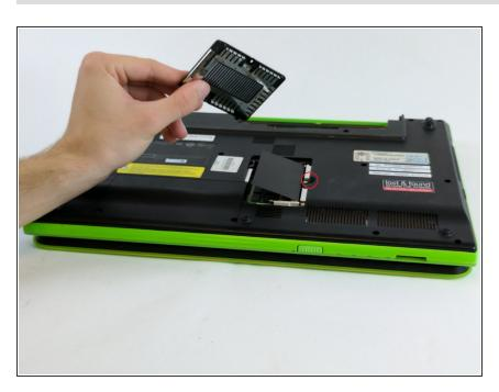
After removing the screw, using your finger slowly lift out and remove the cover.
