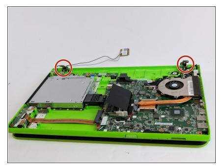
• They are two hinges that hold the screen on. Make sure to pay attention to where the screws come from in order to put them back and to make installation easier.
