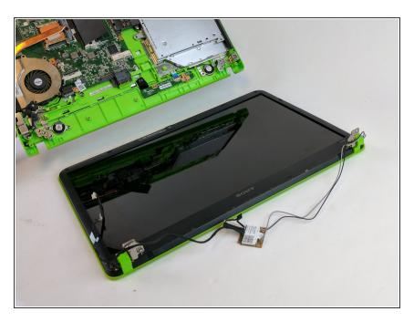
• By folding up the hinges the screen will simply slide away from the body of the computer and you can then put the new screen into place.
