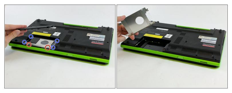
Remove the screws marked in red to remove the hard drive cover and the screws marked in blue to loosen the hard drive. Then gently slide the hard drive out.
