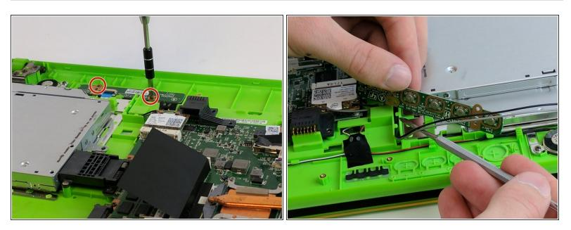
• You will need to unscrew this small circuit board and fold it up to get the wires out from under it.
