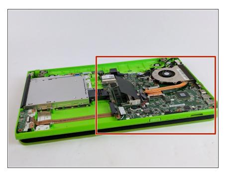
Now that the backing plate is off make sure to be careful of the Motherboard and its components from being damaged. from here on out it is recommended that you wear a anti static bracelet or at the very least touching something metal to remove any static electricity that you may have built up
