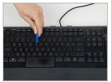
Insert the plastic opening tool underneath the edge of the key.
