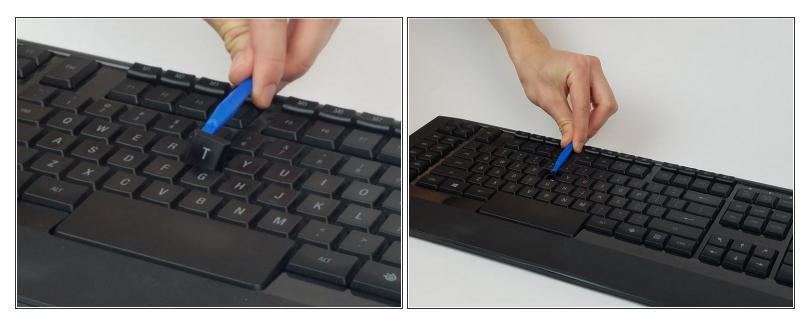
• Gently pry the damaged key with the plastic opening tool at an upward angle.
