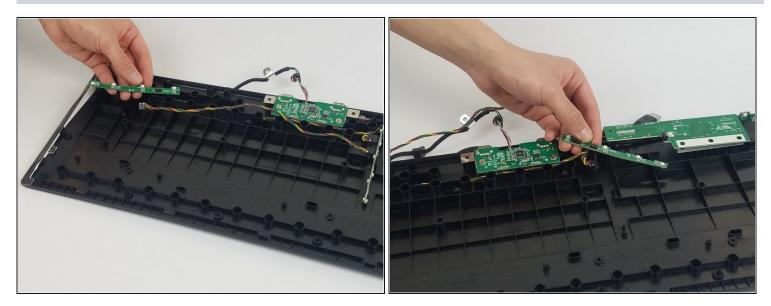
Remove the LEDs.
