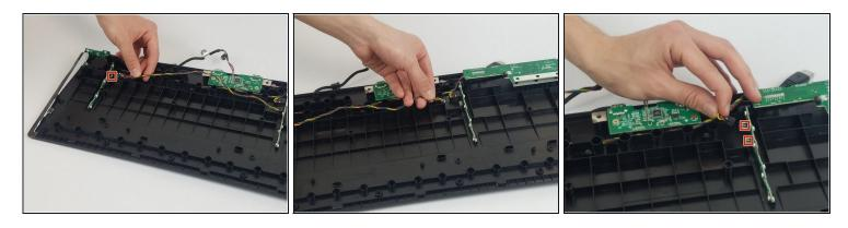
Unplug the wires connected to the LEDs.
