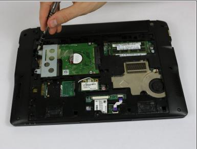
Using the JIS J1 Screwdriver Bit and Driver, remove the two screws (9.0 mm) from the outward side of the hard drive.
