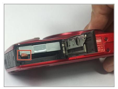
• Depress the orange lever holding the battery in place to unlock it.
