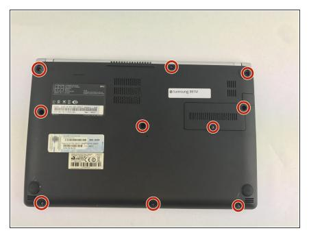
Remove the ten 4mm screws located on the back of the laptop with a PH0 screw bit, and remove the back cover.
