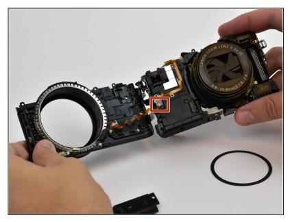
Separate the front cover and focus ring assembly from the front of the camera. Use a plastic spudger to detach the ZIF connector holding the ribbon cable connected to the focus assembly.
