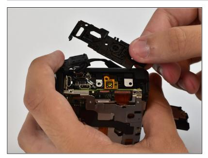
Remove the USB/HDMI panel from the right side of the camera.
