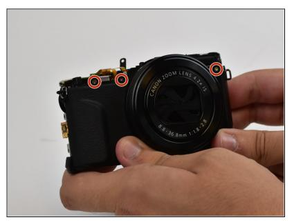
Use a Phillips #000 screwdriver to remove two 3mm screws on the left and one 5mm screw on the right from the front panel.
