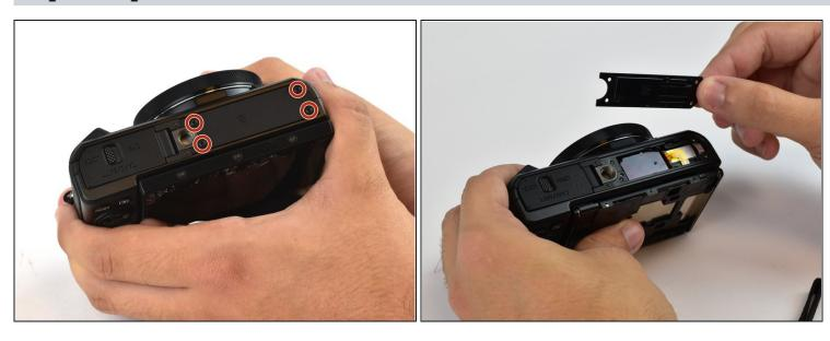
• Use a Phillips #000 screwdriver to remove four 4mm screws from the NFC panel cover on the bottom of the camera.
