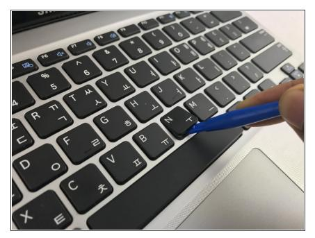
Select the key you would like to remove then slide the plastic opening tool beneath it until you hear a pop.
