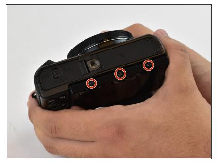
Use a Philips #000 screwdriver to remove the three 2mm screws on the bottom of the LCD screen.
