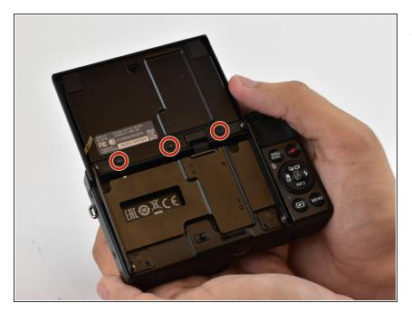
Tilt the LCD screen all the way up and use a Phillips #000 screwdriver to remove the three 4mm screws from the back of the LCD screen.
