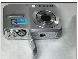
Placing your thumb on the battery cover, push outwards, away from the camera in the direction the arrow is pointing. If done correctly when it's completely unhooked, the latch will open.
