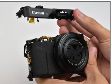
Pry the top cover button assembly off of the camera body by detaching clips around the base of it.
