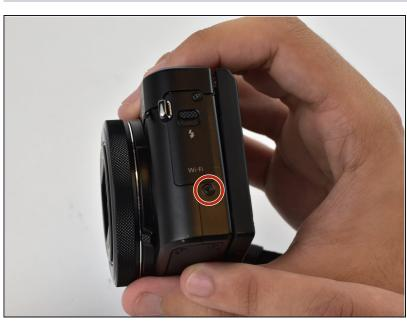
• Use a Phillips #000 screwdriver to remove one 3mm screw on the left of the camera.
