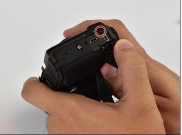
• Use a Phillips #000 screwdriver to remove one 3mm and one 4mm screw on the surface of the right face of the camera, and one under the USB/HDMI cover.
