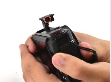
Use a Phillips #000 screwdriver to remove two 3mm screws on the pop-up flash.
