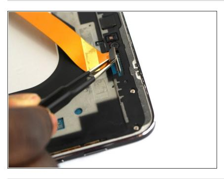
Using the precision tweezers, remove the small press-fit connector from the body of the tablet.
